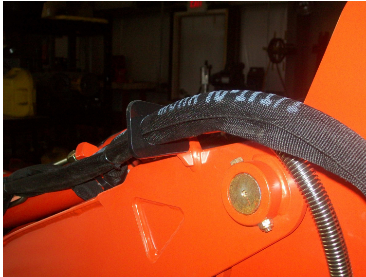
Figure 10 Hose Guides Mounted at the Top of the Backhoe Boom.
