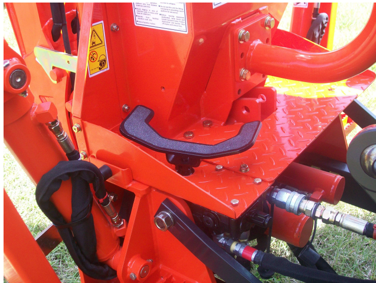
Figure 7 Foot Pedal Installed on LHS of Operator Platform.
